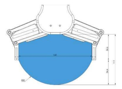
Gripping on long objects can unintentionally activate the Safety switches. The maximum workpiece height (calculated from the end of the fingertips) is dependent on the gripping width (w). For various width values the height (h) limit is given below:
