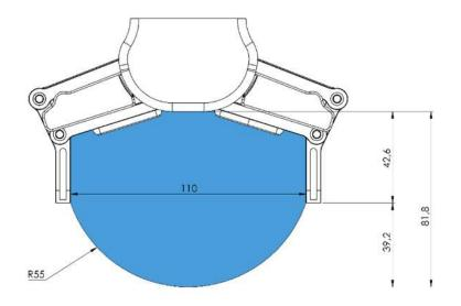
Gripping on long objects can unintentionally activate the Safety switches. The maximum workpiece height (calculated from the end of the fingertips) is dependent on the gripping width (w). For various width values the height (h) limit is given below:
